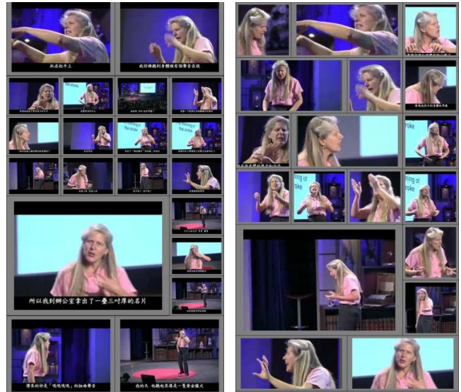
Figure 1. Illustration of baseline (left) and proposed method (right). Applying existing video summarization technique directly on mobile interface which has very limited space may results in some problem. Imagine that putting a huge collage of a video into a smart phone: low zoom level makes the frames unclear, while high zoom level images will occupy lots of spaces.
