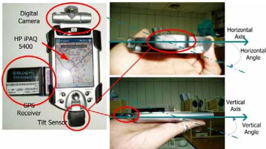
**Figure 5: The HP iPAQ 5550 with camera, GPS receiver, and a Tilt sensor**
