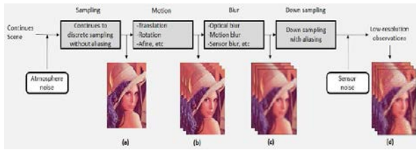
Fig. 2: The observation model of an imaging system relating a high-resolution image to the low-resolution observation frames [12].
