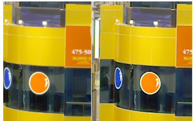
Figure 3: The left picture is original image; the right picture is after unsharp mask function with halo artifact.
