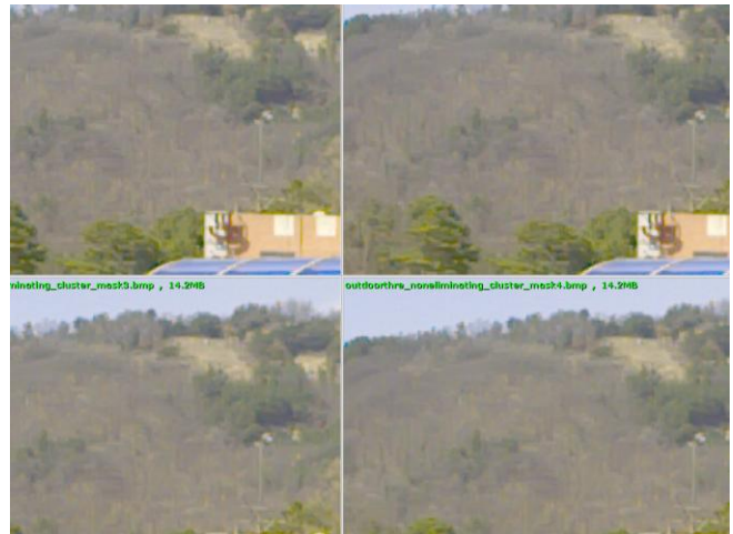
Figure 6: This figure shows that different masks will affect how to catch edge pixels in test image. The left upper picture is the larger mask; the right lower picture is the smaller mask.
