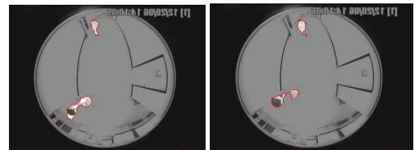
Fig. 9. Edges in gray image are too obscure to locate, which cause the extracted objects to be broken.
