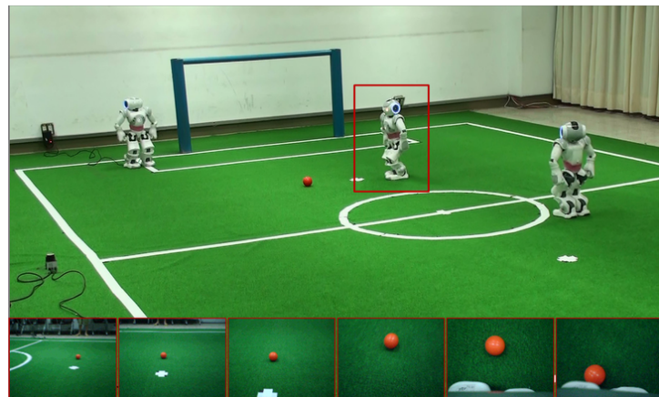
Fig. 2 The Ball Gazing Case: the robot indicated by the red rectangle only detects the ball without any map feature. The bottom images are a sequence of images captured during the task.
