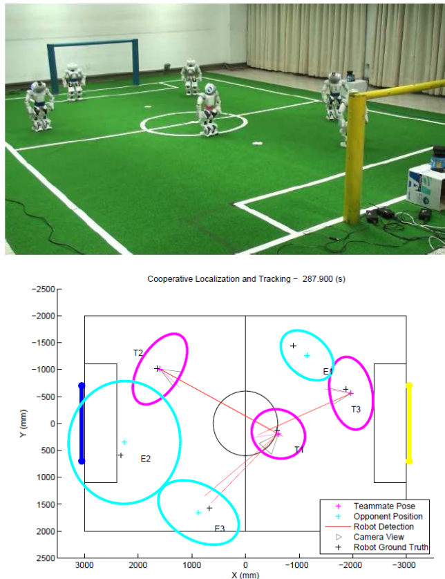
Fig. 8 An example result of CLAT, where three teammate robots and three opponent robots are correctly estimated.
