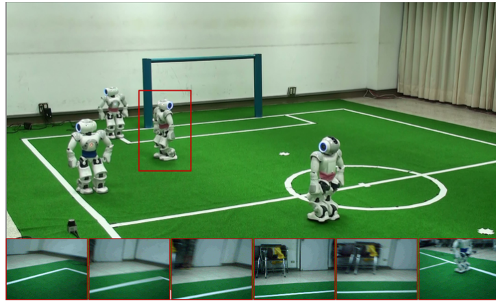
Fig. 1 The Boundary Case: the robot indicated by the red rectangle detects only one field line and two corners. The bottom images are a sequence of images captured during a right to left head motion in 2 seconds.
