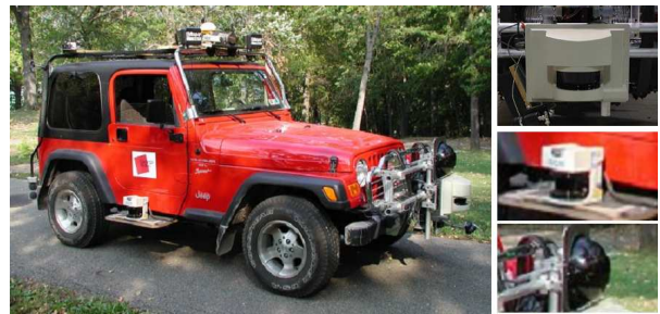
Fig. 1. The Navlab11 vehicle. From the top right to the bottom right: SICK LMS221 laser scanner, SICK LMS291 laser scanner and the tri-camera system.
