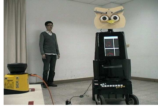
(a) The NTU-PAL2 robot, a person and a SICK S200 laser scanner.
