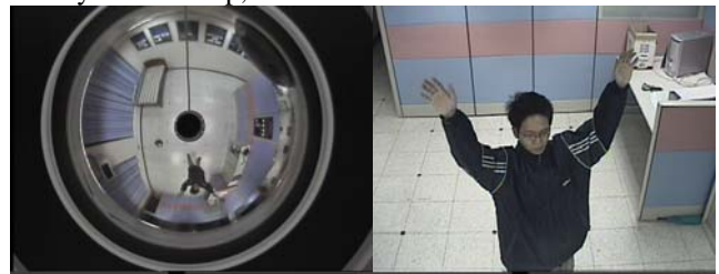
Figure 1. A commercial surveillance system uses the overview+detail interface. (the left is a contextual overview of a scene, and the right is a detailed view)
