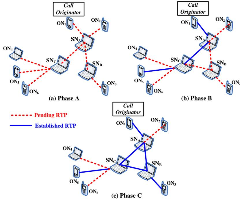
Figure 3: Three Phases for Call Establishment
