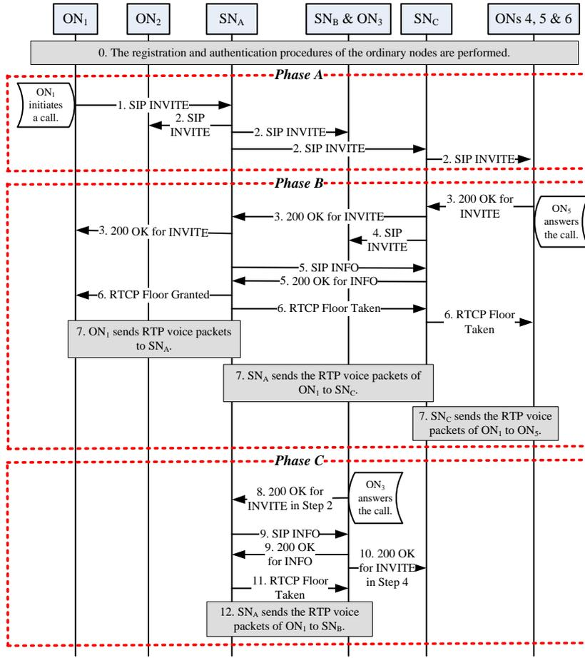
Figure 2: The Detailed Steps for Call Establishment
