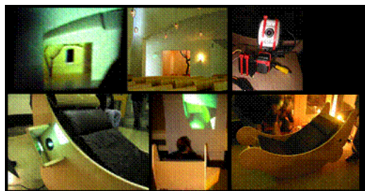
Figure 3. Window Seat rocking chair's up/down and left/right motion controls a remote camera.
