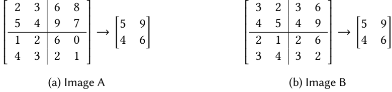
Fig. 2. An illustration of max pooling to extract translational invariance features. The image B is derived from shifting A by 1 pixel in the horizontal direction.
