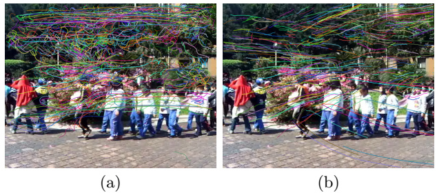
Figure 2: Visualization of feature trajectories (of the children sequence). (a) A frame from the left video, overlapped with its extracted feature trajectories before stabilization: these trajectories twist around in the video volume. After stabilization, feature trajectories become smoother in the transformed video volumes (b). Once trajectories become smooth, the transformed video sequence looks stabilized.
