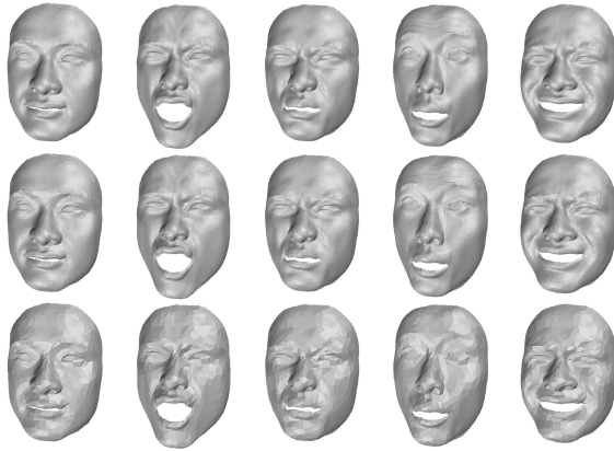
Figure 14: A facial expression animation with 192 frames. Top: The original sequence with 23,725 vertices and 46,853 faces. Middle: 3,201-vertices and 5,825-faces approximation using DOD+DCU approach. Bottom: 1,200-vertices and 1,874-faces approximation.
