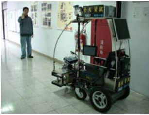
(a) A PTZ camera and a web camera are used for recognizing hand postures.
