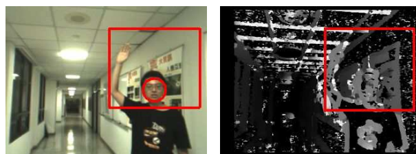
(a) Face detection using single camera (b) Upper body localization using stereo cameras
