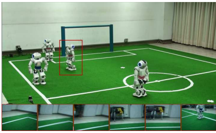
Fig. 2. The Boundary Case: the robot indicated by the red rectangle only detects one field line and two corners. The bottom images are a sequence of images captured during a right to left head motion (in 2 seconds).
