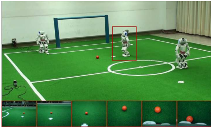
Fig. 3. The Ball Gazing Case: the robot indicated by the red rectangle only detects the ball without any map feature. The bottom images are a sequence of images captured during the task.
